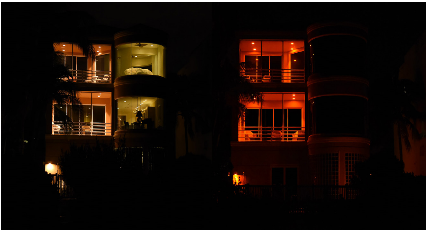
STC retrofitted the lights on Mark and Jill's Hickory Boulevard home with long wavelength amber LEDs and shielded fixtures.
